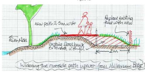
Figure 16. Sketch section through widened flood bank, with options of building the Greenway behind the bank
