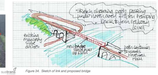
Figure 34. Sketch of link and proposed bridge
