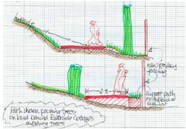
Figure 22. Sketch cross section showing path and screening to railway cottages
