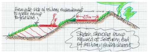
Figure 25. Sketch of ramp from railway and link to Reservoir
