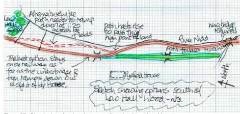
Figure 57. Sketch plan of options between railway level and riverside
