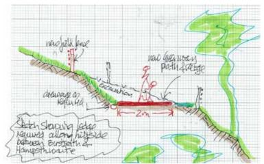
Figure 84. Sketch of section of hillside approaching bridge on the downstream side
