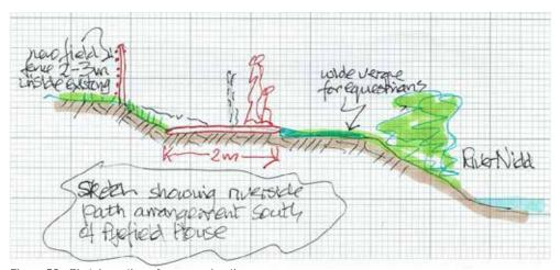
Figure 58. Sketch section of proposed path
