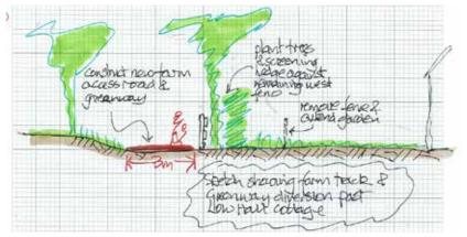
Figure 51. Sketch showing a possible arrangement so as to enhance the privacy of the existing cottage
