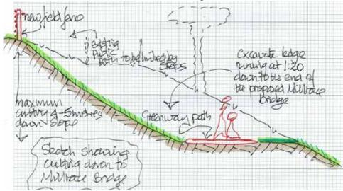
Figure 82. Sketch section showing cutting down to Millrace Bridge
