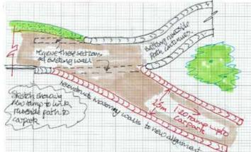
Figure 20. Sketch plan of ramp
