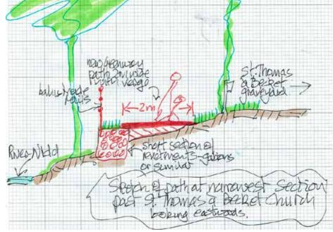
Figure 88. Sketch of path at narrowest section
