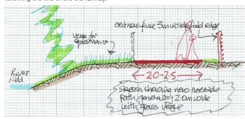
Figure 31. Sketch through typical riverside path section
