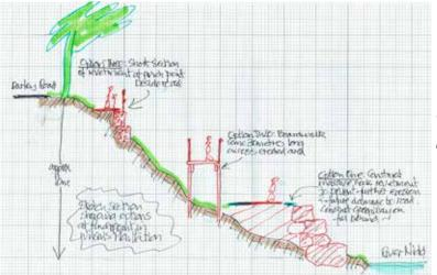
Figure 72. Sketch through option at pinch point
