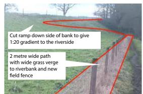
Figure 32. View of bank with overlay showing arrangement of ramp
